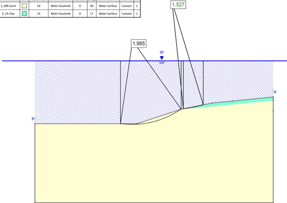
Figure 2- Shallow failure surfaces in very loose and loose sand layers (1V:3H Slope)
