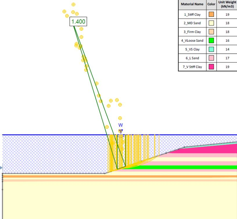
Figure 3 - Factor of Safety < 1 for very soft clay at 1V:3H slope
